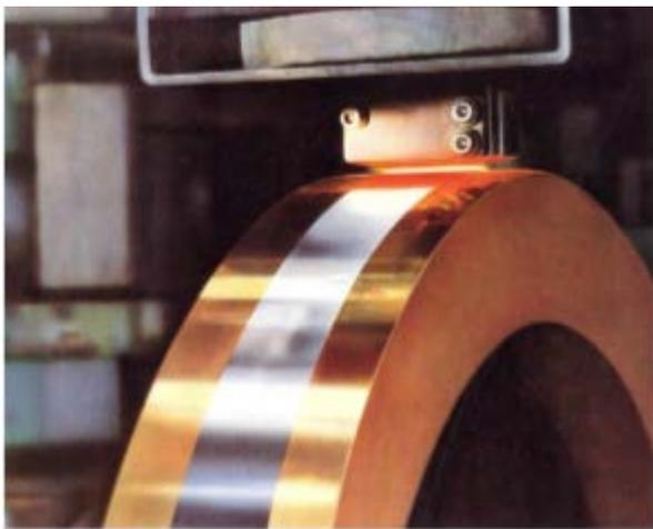
Figure 4: Melt spinning process
