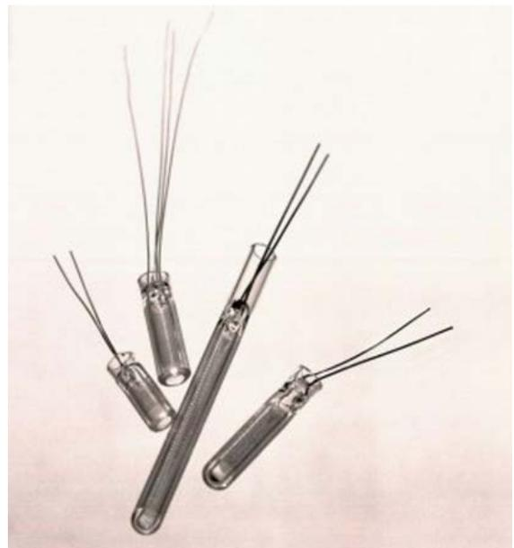
Figure 1: The patenting of the “electrical resistance thermometer made of platinum wire” by W. C. Heraeus in 1906 marks the beginning of modern temperature measuring technology. The novel design (platinum wire wound up on a piece of quartz glass and protected by a quartz glass tube) permitted the safe, accurate and fast measuring of high temperatures.
