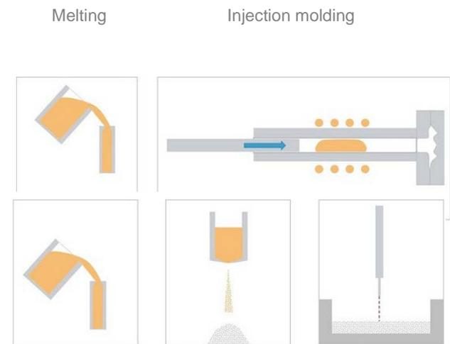
Injection molding has the advantage of enabling 24/7 high-volume production in an automated process. It can be used as an alternative to mechanical machining or metal injection molding.
