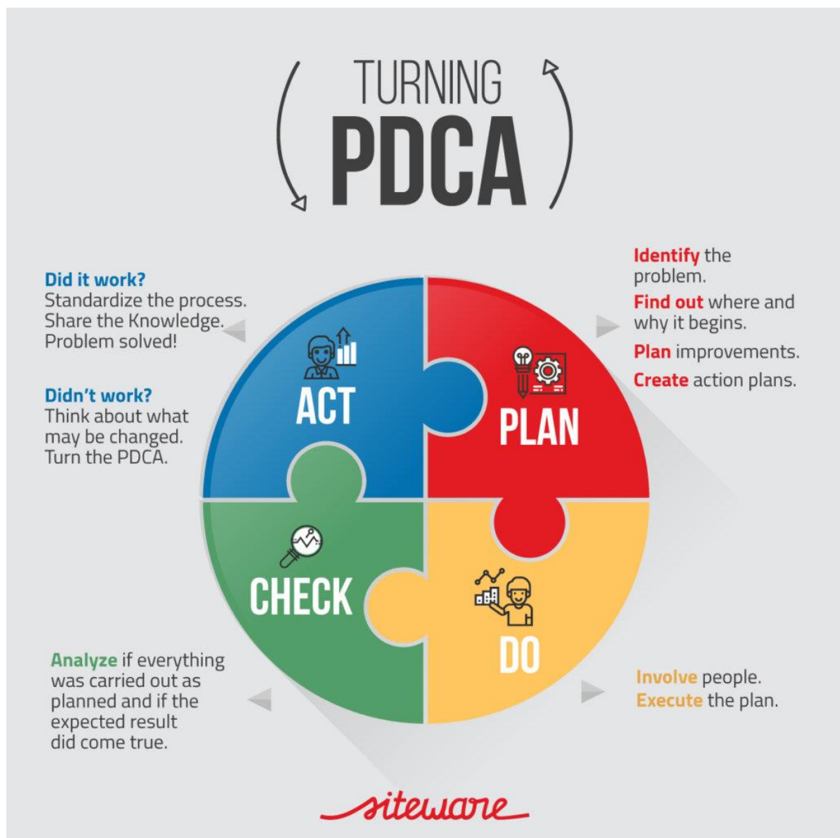
Figure 7: Overview of the processes of the PDCA cycle. Source: https://www.siteware.co/en/methodologies/how-to-do-pdca-step-by-step/
